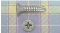
#8 x 3/4" T-2 #2 PFH. All-300 series stainless with Dyna-Coat® .
