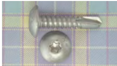
#12 x 1" T-3 #25 torx drive truss head all-300 series stainless with Dyna-Coat® .
