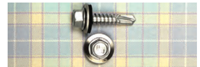
#12 DIA. T-3 HWH #12 dia. 5/16" HWH with or without stainless sealing washer. Choose 1", 1 1/2" or 2".
