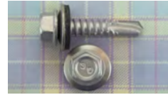
#12 x 1" T-3 #25 torx drive truss head all-300 series stainless with Dyna-Coat® .
