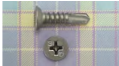
#10 x 3/4" T-3 #2 PFH with undercut all-300 series stainless with Dyna-Coat® .
