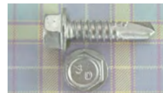
#14 x 1" T-3 #30 torx drive truss head all-300 series stainless with Dyna-Coat® .
