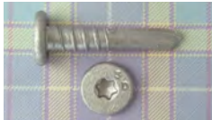
#12-11x1" T-4 #25 torx pancake head clip screw all-300 series stainless with Dyna-Coat® .
