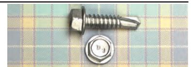
#14 DIA. T-3 #14-14 T-3 3/8" HWH. With or without S/S washer. Choose 1", 1 1/4", 1 1/2", 2", 3", 4", 5", 6" or 8".
